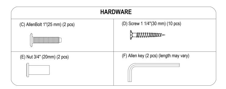
Do not fully tighten all bolts until all parts are in place. (please add an extra 1/2 revolution to the bolts when using spring washer after tightening)
