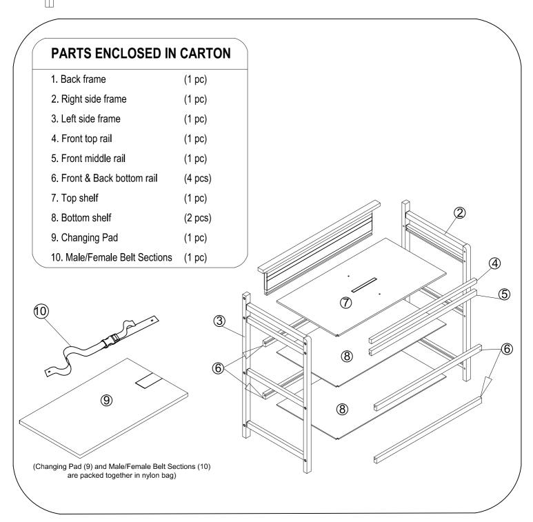
Do not fully tighten all Screws until all parts are in place.
