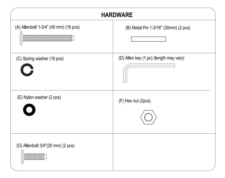
Do not fully tighten all bolts until all parts are in place. (please add an extra 1/2 revolution to the bolts when using spring washer after tightening)
